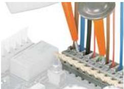
Testing with test probes.
