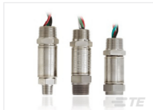
TE Part #11108663-00 300 PSI, 1/4MNPT, 4-20mA, Conduit, 18AWG
