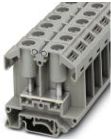
Universal terminal block with bolt connection, cross section: 0.1 - 25 mm 2 , width: 18 mm, color: gray
