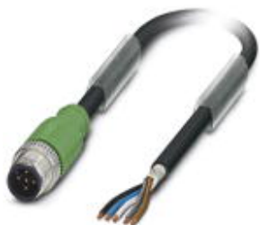
Sensor/Actuator cable, 5-position, PUR halogen-free, black-gray RAL 7021, shielded, Plug straight M12, A-coded, on free cable end, Cable length: 1.5 m
