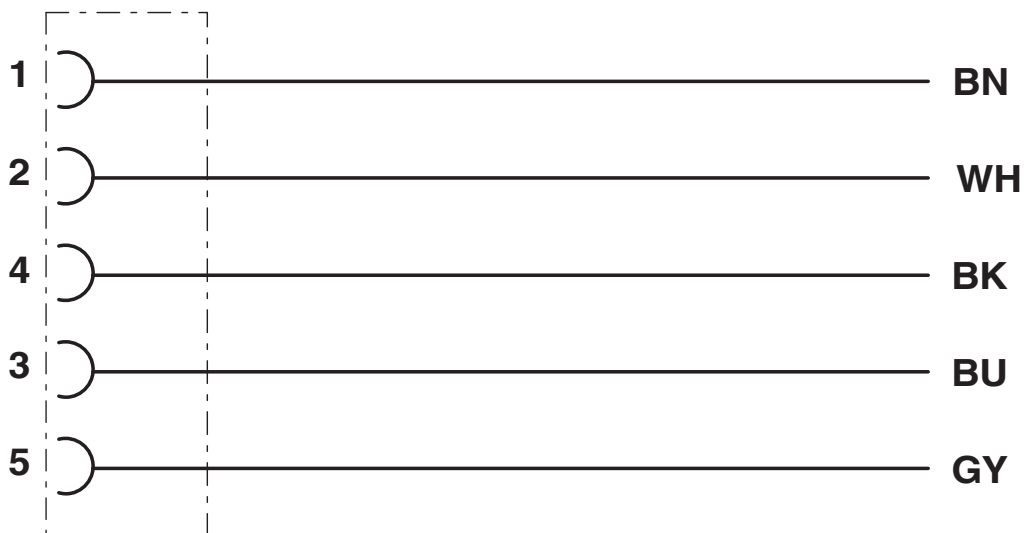
Contact assignment of the M12 socket
