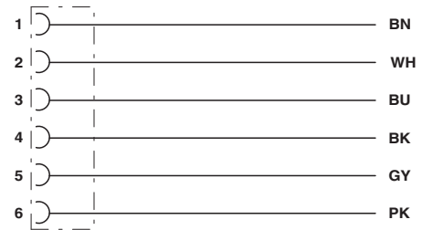
Contact assignment of the M12 socket
