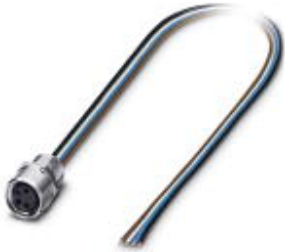
Sensor/actuator flush-type socket, 4-pos., M8, front/screw mounting with M8 thread, with 0.5 m PVC litz wire, 4 x 0.25 mm 2
