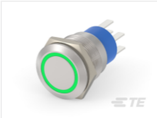
TE Part #5-2213767-3 AV19 DPM 3A MOVE RING LED GREEN 12V
