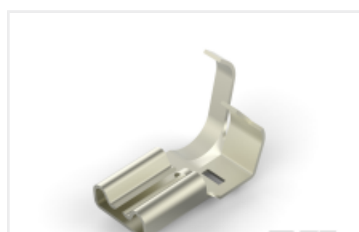
TE Part #2238197-3 250 FASTON,FLAG,REC.,18-12 AWG, TPBR
